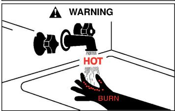
Water temperature over 52°C (125°F) can cause severe burns instantly or death from scalds.
